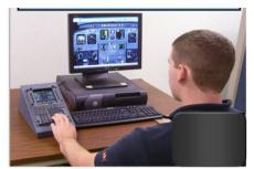
Figure 6. FMS Handset & Simulated FMS Program
